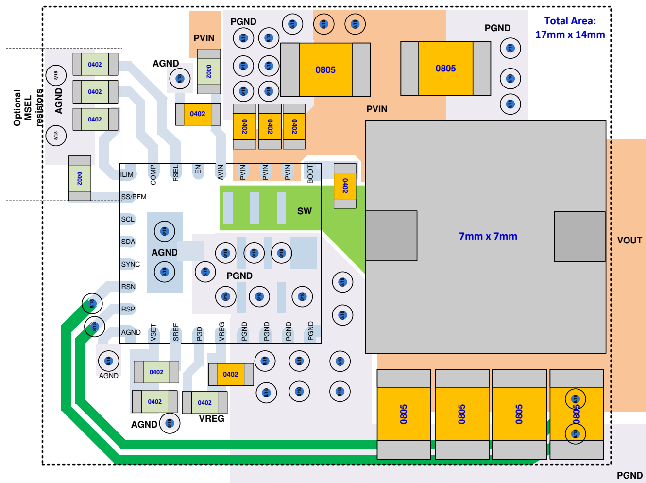
Figure 10-1. Example PCB Layout
