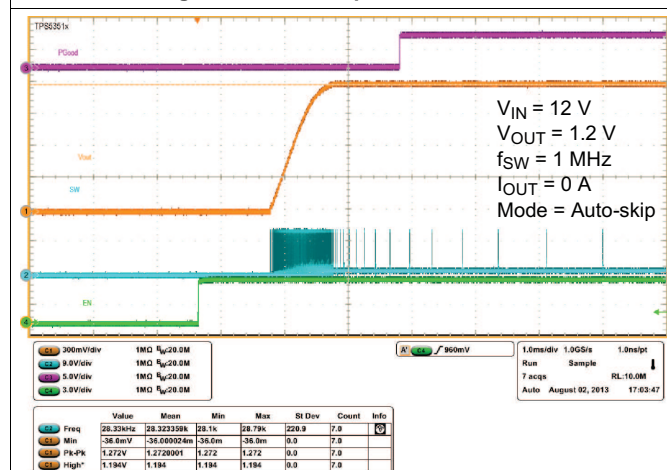
Figure 19. Auto-Skip Mode Load Transient
