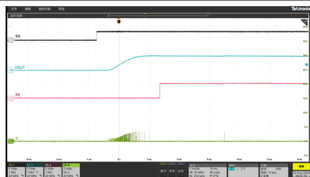
Figure 8-6. Start-Up Relative to EN Rising, Iout = 0A, PSM Mode
