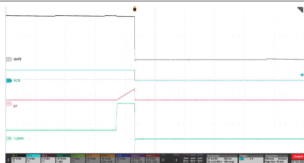
Figure 9-9. \text{I}^2\text{T} based Overcurrent Response of TPS4812-Q1 EVM for 6A to 23A Load Step
