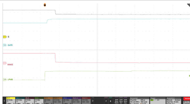
Figure 9-6. State Transition From LPM to Active Mode ( \overline{\text{LPM}} = Low to High, V_{\text{IN}} = 48V, No Load)
