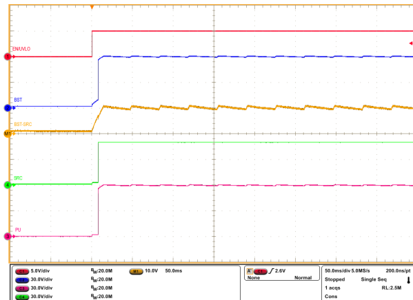
Figure 8-3. Start-Up Profile of Bootstrap Voltage with INP = HIGH and C_{BST} = 470\text{nF}
