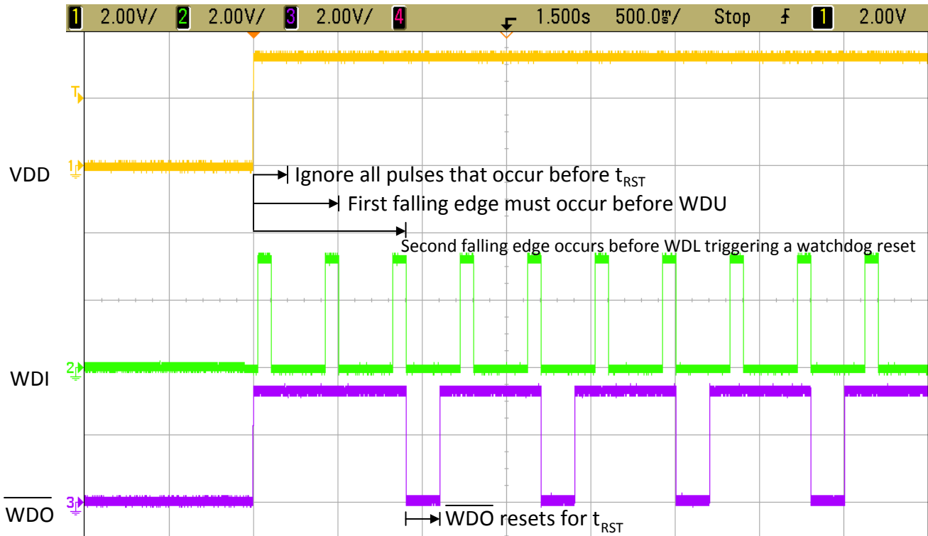
Figure 8-5. Watchdog Fault Caused by WDI Pulse Arriving Too Early (Before t_{WDL}(\min) )
