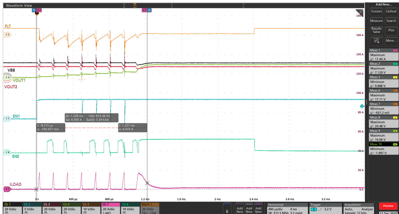
Figure 8-29. 220uF Capacitive Load Charging with Channel 1 of TPS2HC16-Q1 Device at 13.5V VBB, ILIM Pin shorted to ground and 125°C Ambient Temperature (no load on channel 2)
