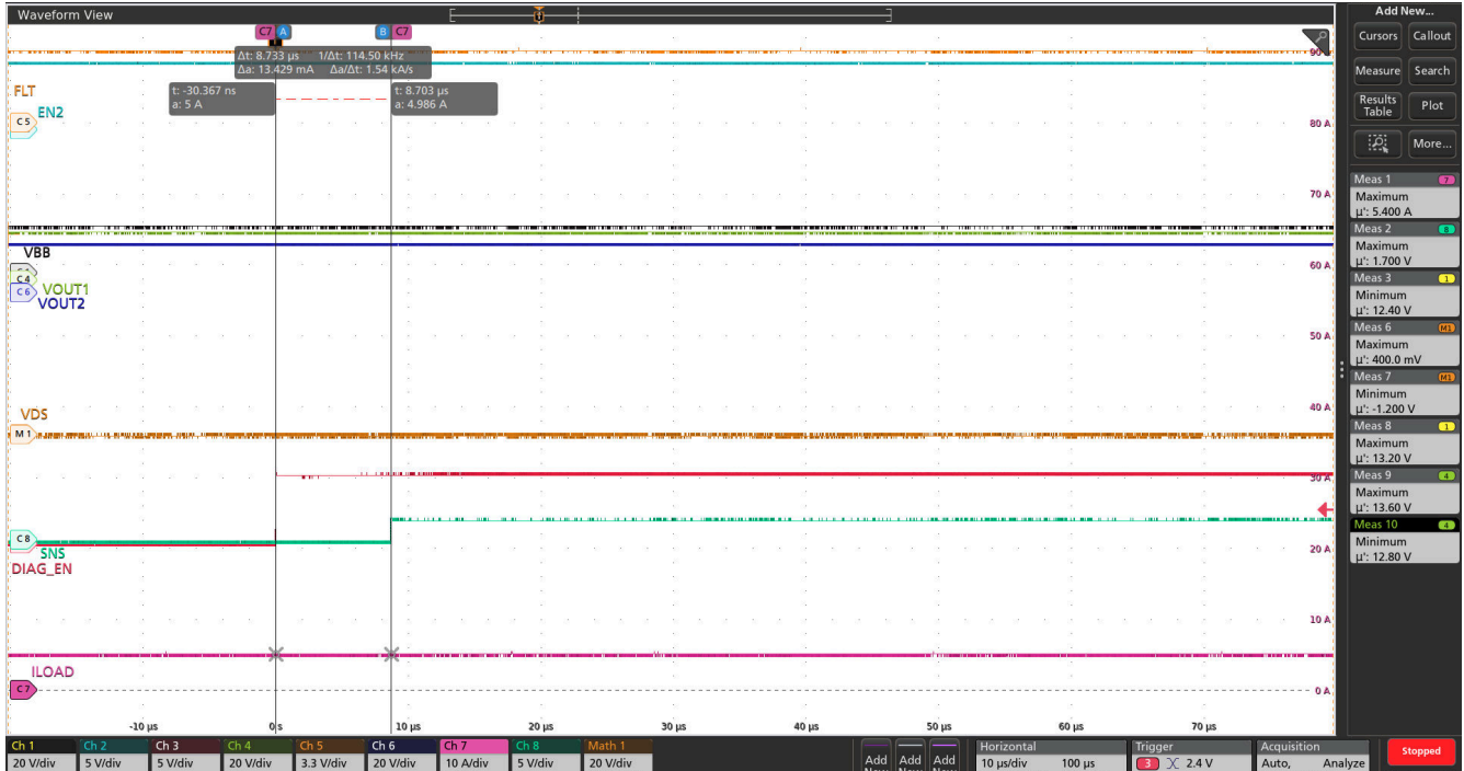
Figure 8-5. SNS Response Time with DIAG_EN ( t_{SNSION1} )
