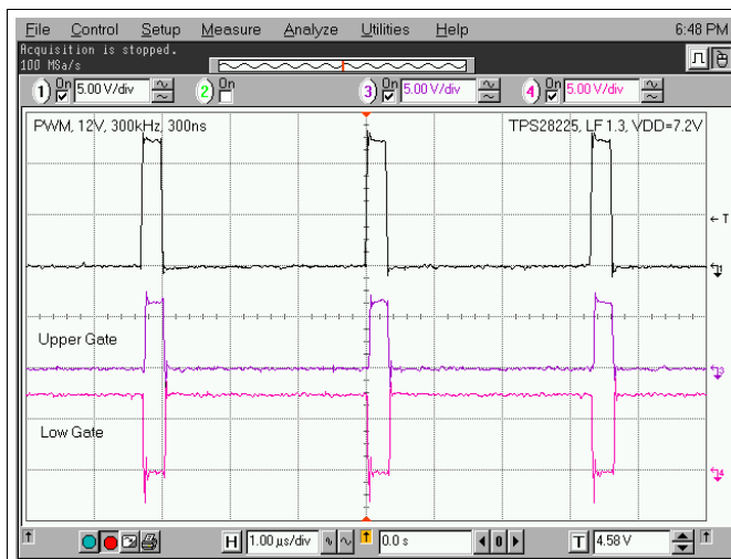
Figure 23. 12-V PWM Pulse at V_{DD} = 7.2 V
