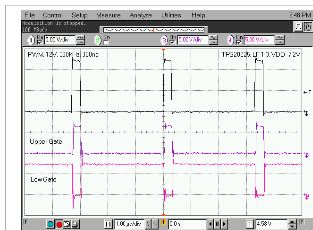
Figure 7-4. 12-V PWM Pulse at V_{DD} = 7.2 V
