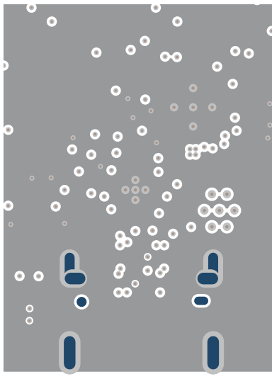
Figure 8-28. TPS26750 PCB Layout - GND Layer 2
