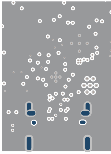
Figure 8-31. TPS26750 PCB Layout - GND Layer 5
