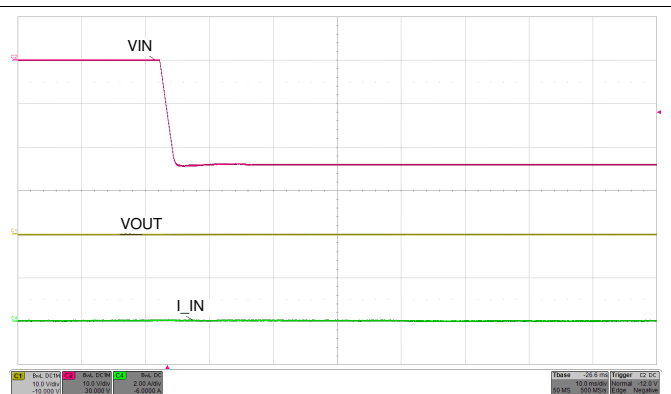
Figure 63. Reverse Polarity Protection
