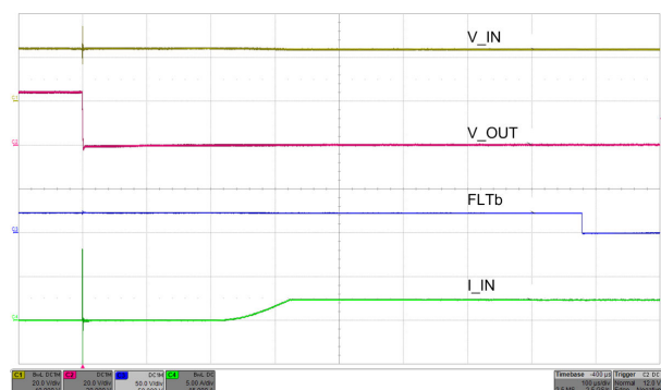
Figure 7-27. Hot-Short: Fast Trip Response and Current Regulation
