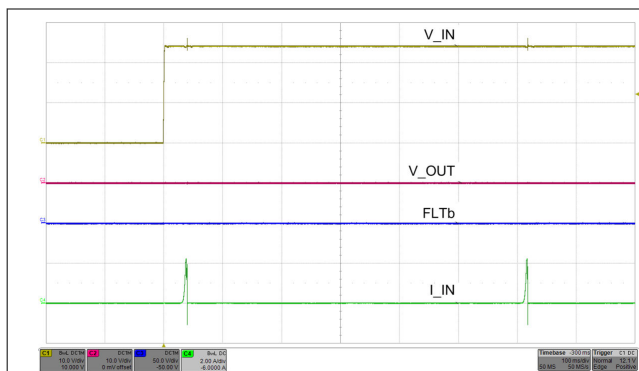
Figure 10-13. Turnon With Short Circuit on Output
