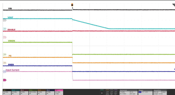
Figure 7-37. Power Down Using PMBus Command
