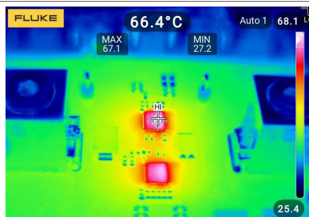
Figure 9-14. One (1) TPS25990 eFuse and one (1) TPS25985x eFuse in Parallel: Temperature Rise with 110-A DC Current at Room Temperature (No Air-Flow)
