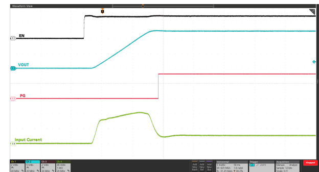
Figure 9-6. Start-up with EN/UVLO: V_{IN} = 12 V, EN/UVLO Stepped Up From 0 V to 3 V, C_{LOAD} = 50 mF, R_{LOAD(Start-up)} = 0.48 \Omega , C_{DVRT} = 33 nF, V_{IREF} = 1 V, R_{ILIM(TPS25990)} = 422 \Omega , and R_{ILIM(TPS25985)} = 316 \Omega
