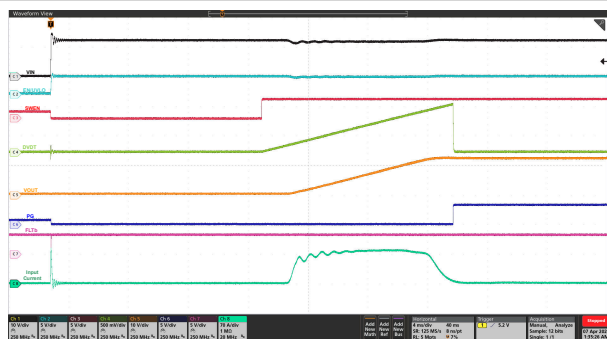
Figure 9-4. Input Hot Plug: V_{IN} Stepped Up from 0 V to 12 V, C_{LOAD} = 55 mF, C_{DVRT} = 33 nF, R_{IREF} = 40.2 k \Omega , and R_{ILIM} on Each Device = 300 \Omega
