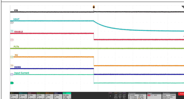
Input supply held steady, EN/UVLO pin toggled from high (above V_{UVLO(R)} ) to low (below V_{SD(F)} )
