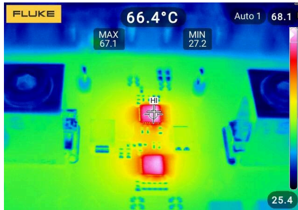
Figure 8-12. Two Devices in Parallel Temperature Rise with 110-A DC Current at Room Temperature (No Air-Flow)
