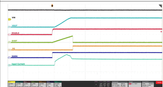
C_{OUT} = 15.5\text{ mF} , R_{OUT} = 0.6\ \Omega , C_{dVdt} = 33\text{ nF}
