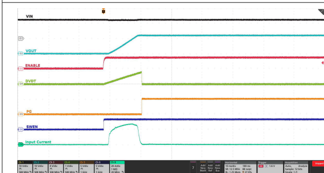
C_{OUT} = 18\text{ mF} , C_{dVdt} = 33\text{ nF}
