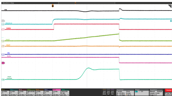
Figure 8-8. Power Up into Short: V_{IN} = 12 V, EN/UVLO Stepped Up From 0 V to 3 V, R_{REF} = 40.2 k \Omega , R_{ILIM} on Each Device = 442 \Omega , and OUT Shorted to GND
