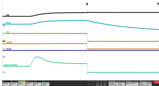
Figure 6-29. Input Overvoltage Protection Response
