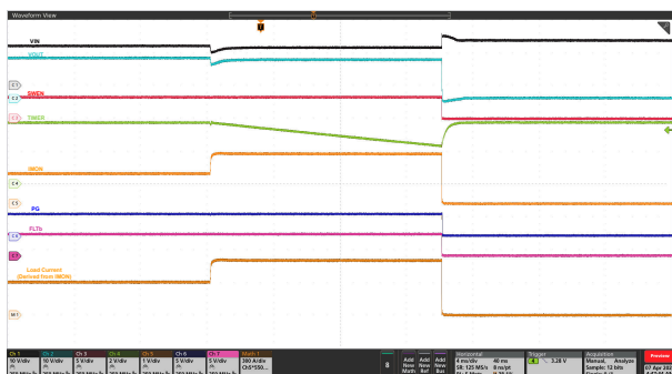
Figure 8-10. Circuit-Breaker Response: V_{IN} = 12 V, C_{TIMER} = 22 nF, C_{LOAD} = 50 mF, R_{IMON} = 200 \Omega , R_{REF} = 40.2 k \Omega , and Load Current Stepped up From 250 A to 400 A for > 20 ms
