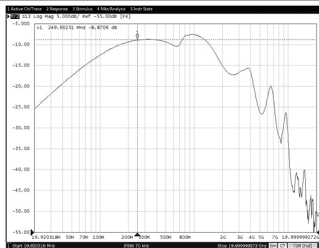
Figure 8-24. Off-state Data-Switch Isolation vs Frequency
