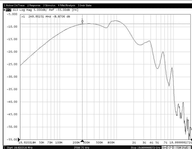
Figure 8-24. Off-state Data-Switch Isolation vs Frequency
