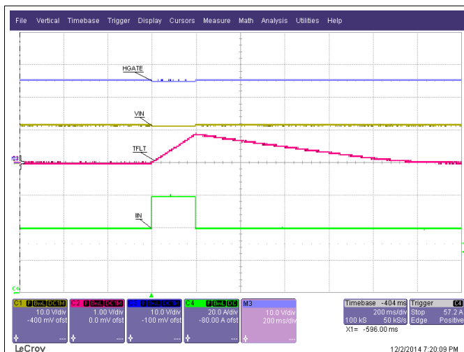
Figure 54. 60A Load Step for 200 ms
