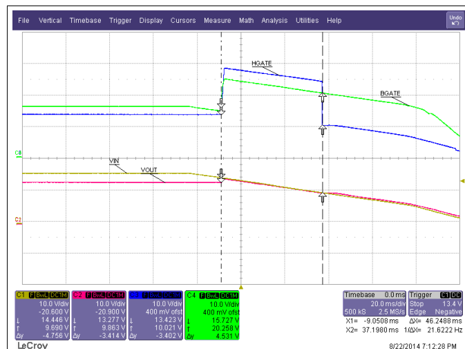
Figure 40. Under/Over Voltage with VIN Falling
