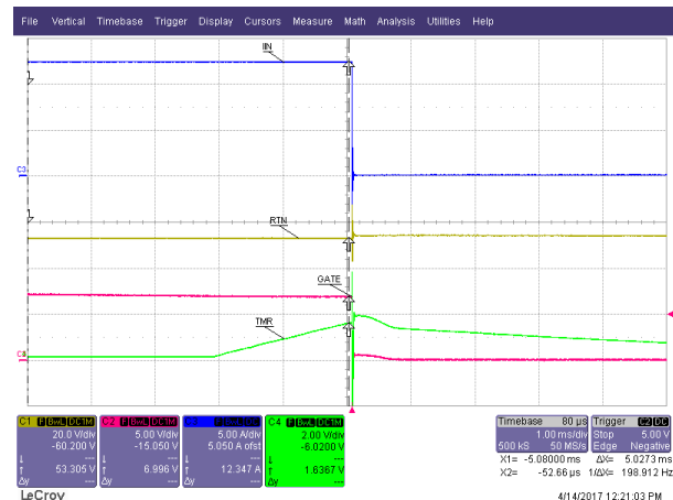
Figure 28. Output Hot Short (VinB = 60 V)
