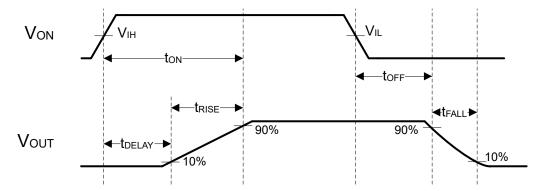
**Figure 8-1. Timing Parameter Measurement Information**
