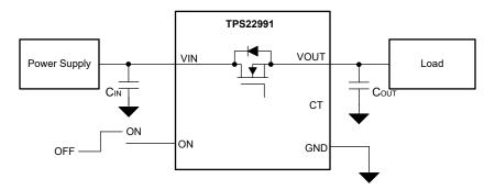
Figure 10-1. Typical Application Diagram
