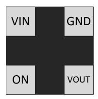
Figure 5-1. TPS22991 RAA Package, 4-Pin UQFN (Top View)
