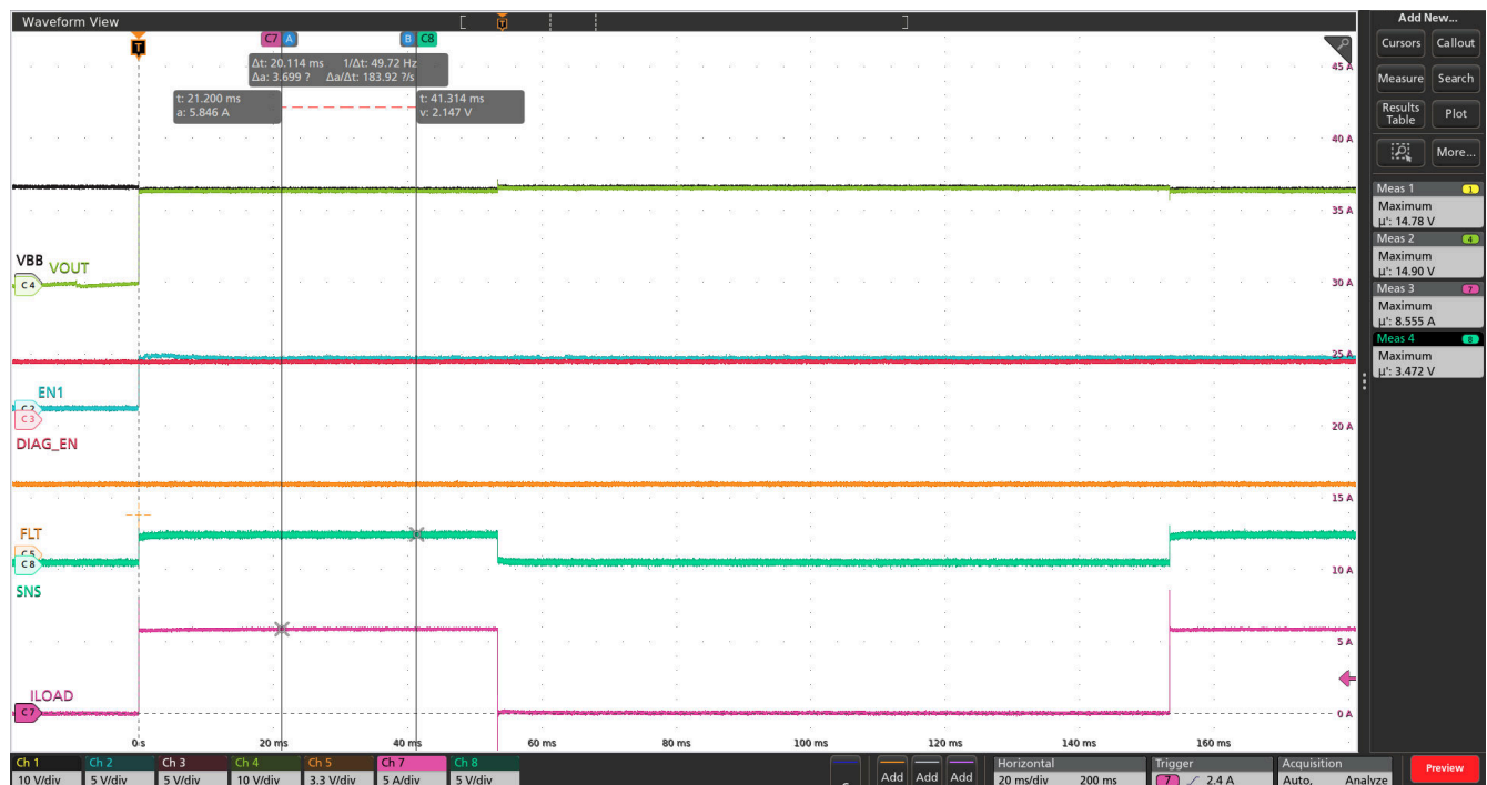
Figure 8-4. SNS Pin Voltage with Varying Load Current ( R_{SNS} = 1k\Omega )
