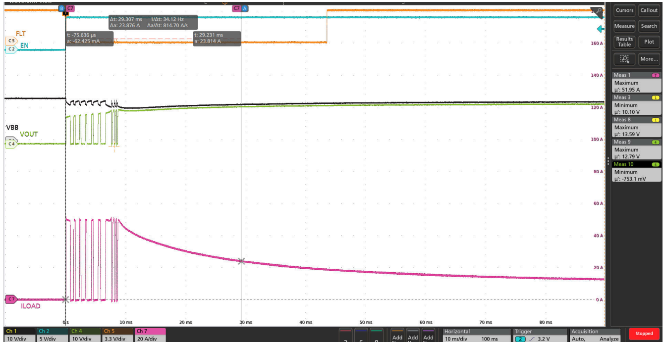
Figure 8-35. 140W Bulb Charging with TPS1HC03-Q1 at 13.5V VBB, T_A (device) = 25°C, T_A (bulb) = 25°C, ILIM = GND
