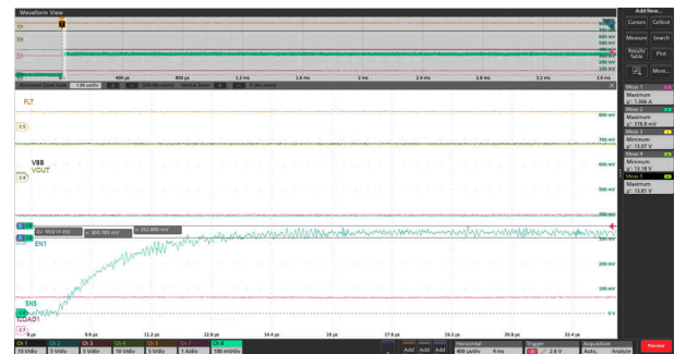
Figure 8-10. SNS Pin Ripple With 150pF C_{SNS} at V_{BB} = 13.5V , I_{LIM} = OPEN , R_L = 10\Omega , R_{SNS} = 1k\Omega and T_A = 25^\circ C
