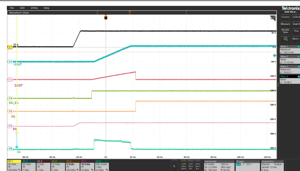
Figure 6-13. Allowed Operating Area (AOA) in Startup
