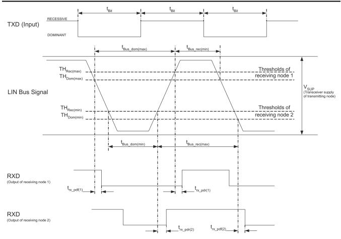
Figure 7-1. Definition of Bus Timing Parameters
