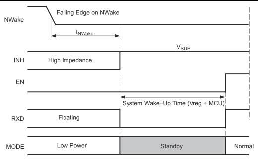
Figure 8-3. Wake-Up Via NWake Timing Diagram
