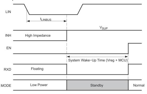
Figure 8-2. Wake-Up Via LIN Bus Timing Diagram
