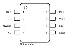
Figure 6-1. D Package, 8-Pin SOIC
