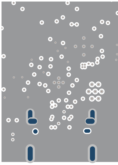
Figure 7-6. TPS26750 PCB Layout - GND Layer 2
