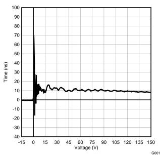
Figure 5. IEC 61000-4-2 Voltage Clamp Waveform 8-kV Contact
