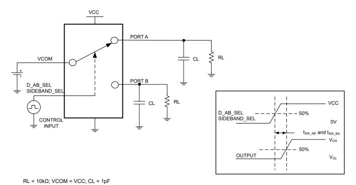
Figure 6-2. Switching Time Between Channels ( $t_{SW\_AB}$  and  $t_{SW\_BA}$ )
