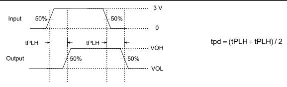
Figure 6-3. Propagation Delay (tpd)
