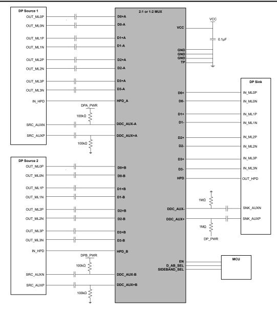
Figure 8-1. Choosing One of Two DisplayPorts - Application Schematic
