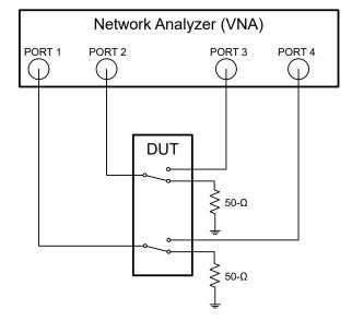
Figure 6-5. Differential Off-Isolation (OISO)
