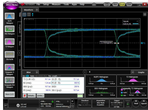
Figure 6-8. Through a Typical TMUXHS221LV Channel at 480Mbps
