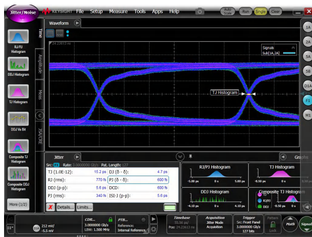
Figure 6-9. Through Calibration Traces at 3Gbps
