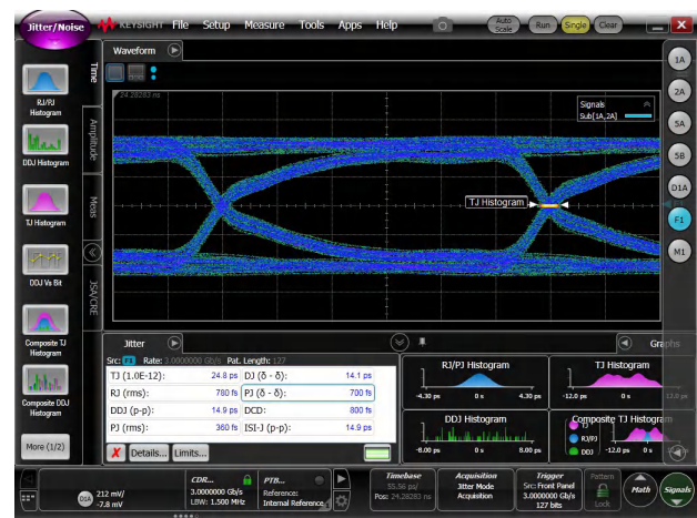
Figure 6-10. Through a Typical TMUXHS221LV Channel at 3Gbps
