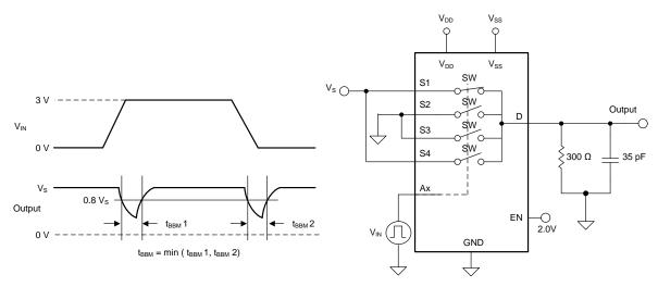
Figure 21. Break-Before-Make Delay Measurement Setup
