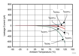
Figure 29. Leakage Current vs Temperature
