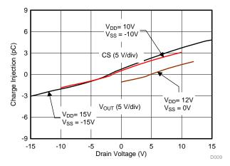
Figure 32. Drain-to-Source Charge Injection vs Drain Voltage
