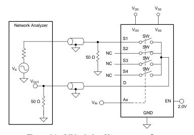
Figure 24. Off Isolation Measurement Setup
