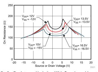
Figure 35. On-Resistance Variation With Supply and Input Voltage
