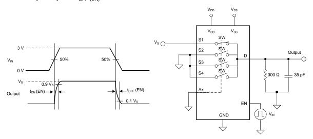
Figure 22. Turn-On and Turn-Off Time Measurement Setup
