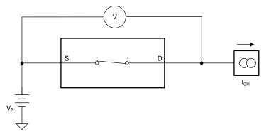
Figure 17. On-Resistance Measurement Setup
