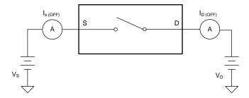
Figure 18. Off-Leakage Measurement Setup
