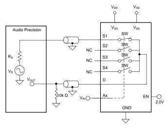
Figure 27. THD+N Measurement Setup
