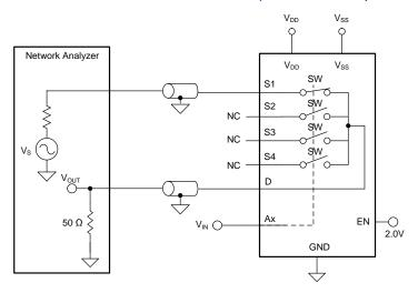
Figure 26. Bandwidth Measurement Setup
