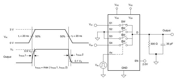
Figure 20. Transition-Time Measurement Setup
