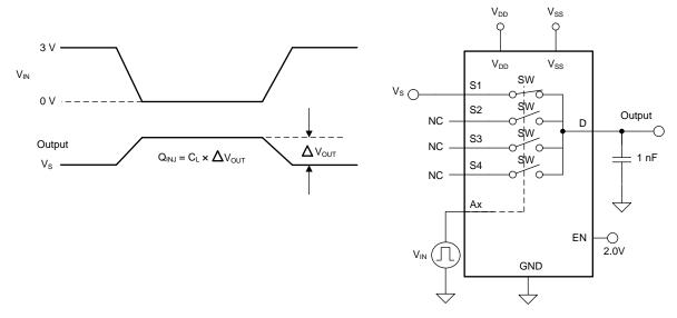
Figure 23. Charge-Injection Measurement Setup
