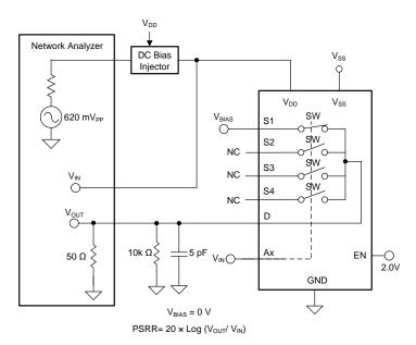
Figure 28. AC PSRR Measurement Setup
