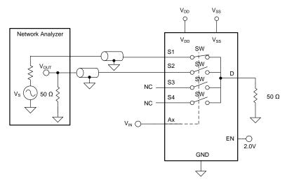
Figure 25. Channel-to-Channel Crosstalk Measurement Setup
