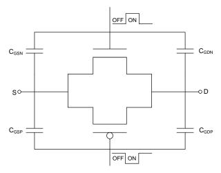
Figure 30. Transmission Gate Topology
