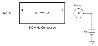
Figure 19. On-Leakage Measurement Setup
