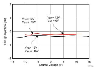
Figure 31. Source-to-Drain Charge Injection vs Source Voltage
