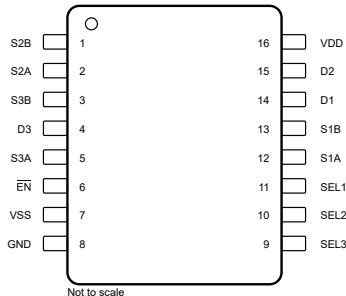
**Figure 5-7. TMUX4053 PW Package, 16-Pin TSSOP
