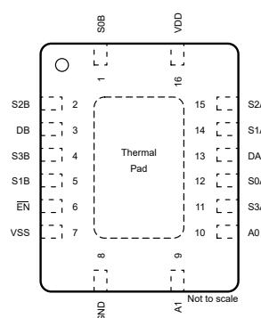
**Figure 5-6. TMUX4052 BQB Package, 16-Pin WQFN (Top View)**
