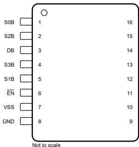
**Figure 5-4. TMUX4052 PW Package, 16-Pin TSSOP
