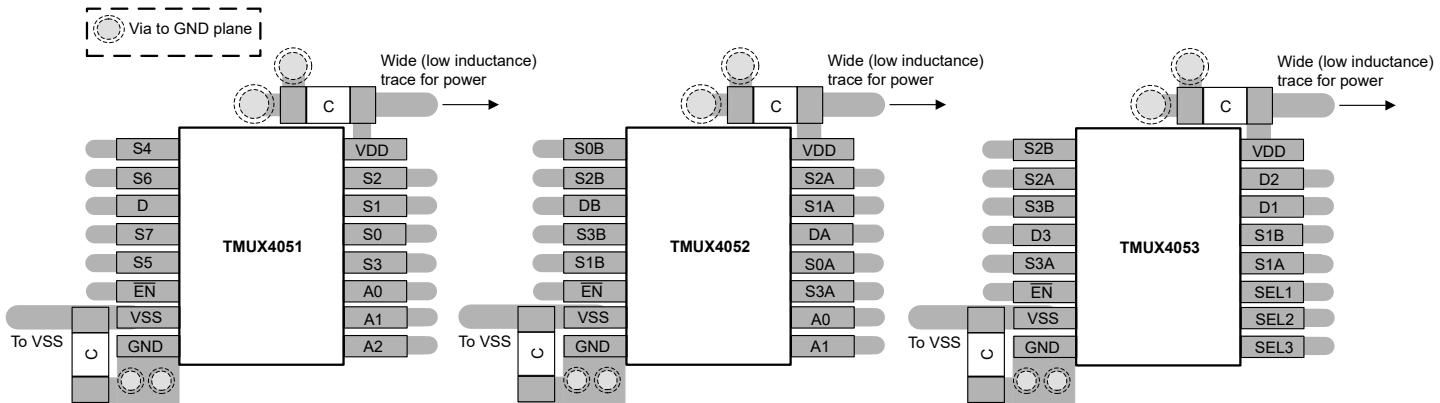
Figure 9-3. TMUX4051, TMUX4052, and TMUX4053 Layout Example
