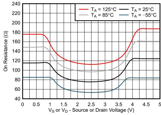
Figure 6-2. On-Resistance vs Temperature
