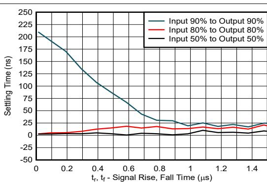
Figure 6-5. System Settling Time
