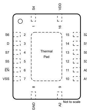
**Figure 5-3. TMUX4051 BQB Package, 16-Pin WQFN (Top View)**
