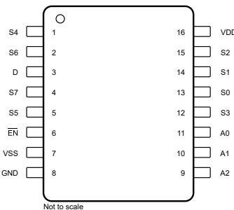
**Figure 5-1. TMUX4051 PW Package, 16-Pin TSSOP (Top View)**
