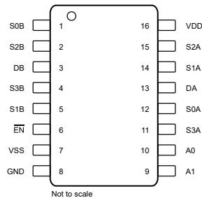
**Figure 5-5. TMUX4052 DYY Package, 16-Pin
