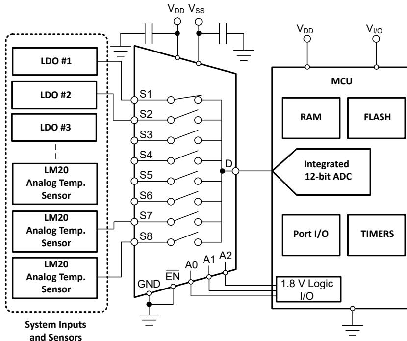
Figure 9-1. Multiplexing Signals to an Integrated ADC with TMUX4051
