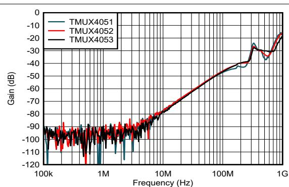
Figure 6-8. Off-Isolation vs Frequency
