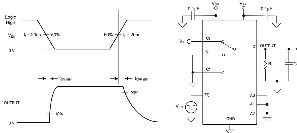
Figure 7-6. Turn-On and Turn-Off Time Measurement Setup
