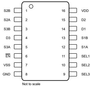
**Figure 5-8. TMUX4053 DYY Package, 16-Pin
