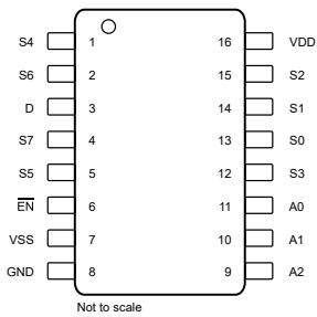
**Figure 5-2. TMUX4051 DYY Package, 16-Pin SOT-23-THIN (Top View)**
