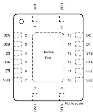
**Figure 5-9. TMUX4053 BQB Package, 16-Pin WQFN (Top View)**
