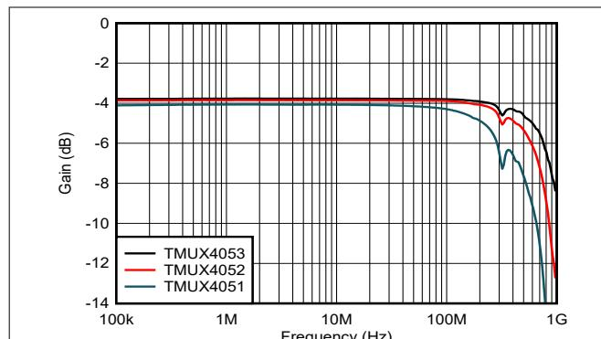
Figure 6-7. On Response vs Frequency
