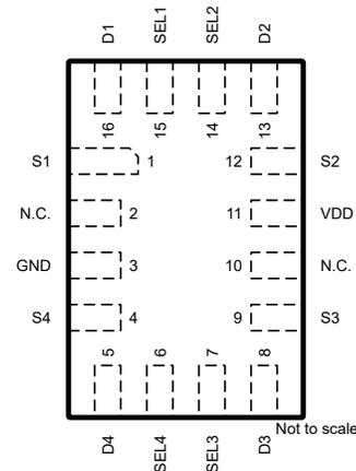
Figure 5-2. RSV Package, 16-Pin UQFN (Top View)
