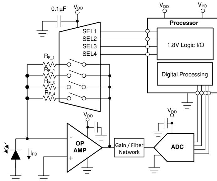
**Figure 9-5. Switching Gain Settings of a TIA circuit**
