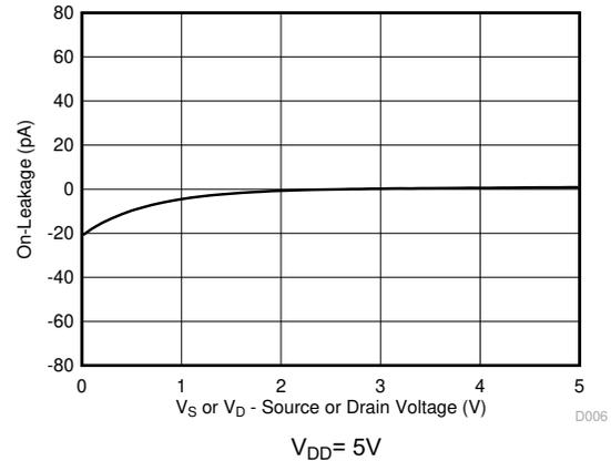
**Figure 9-4. On-Leakage vs Source or Drain Voltage**
