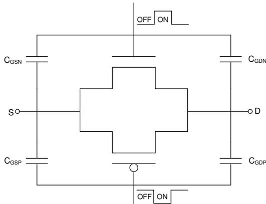
Figure 8-3. Transmission Gate Topology
