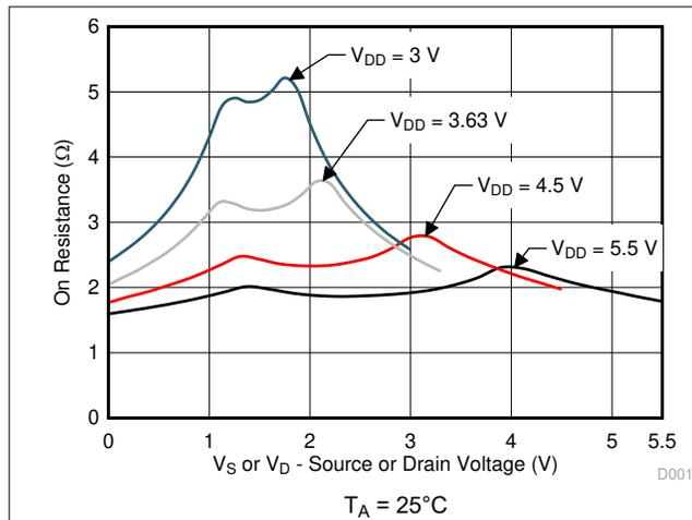
**Figure 6-1. On-Resistance vs Source or Drain Voltage**
