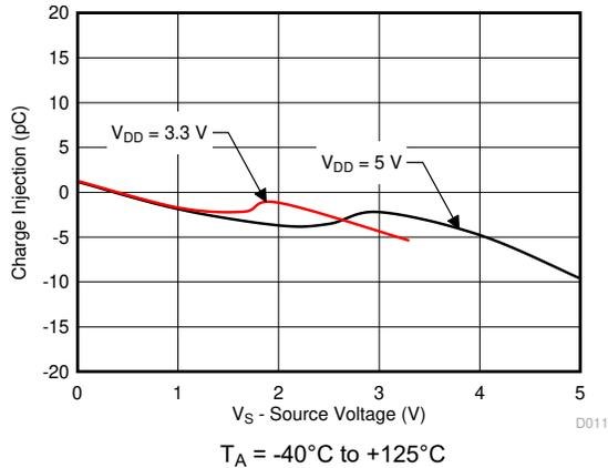
**Figure 9-3. Charge Injection vs Source Voltage**
