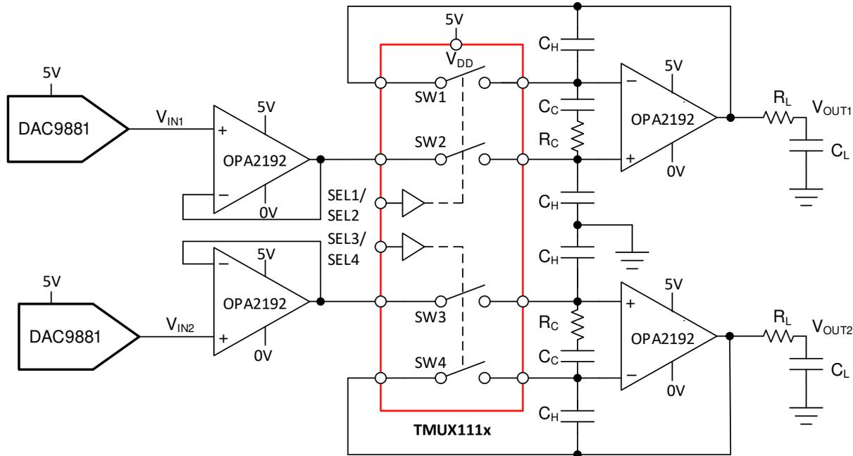
Figure 9-2. 2-Channel Sample-and-Hold Circuit with Pedestal Error Compensation
