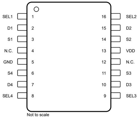
Figure 5-1. PW Package, 16-Pin TSSOP (Top View)
