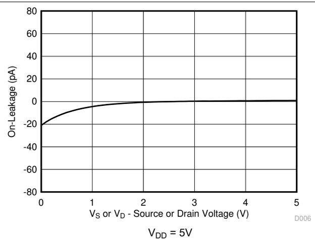
**Figure 6-6. On-Leakage vs Source or Drain Voltage**
