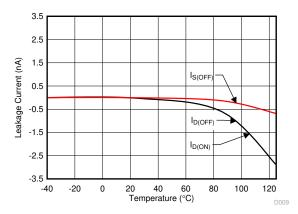
Figure 7-12. Leakage Current vs Temperature
