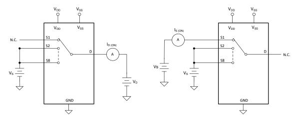
Figure 7-3. On-Leakage Measurement Setup
