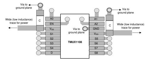
Figure 8-4. TMUX1108 Layout Example
