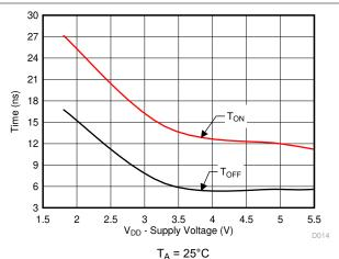
Figure 6-14. T<sub>ON (EN)</sub> and T<sub>OFF (EN)</sub> vs Supply Voltage
