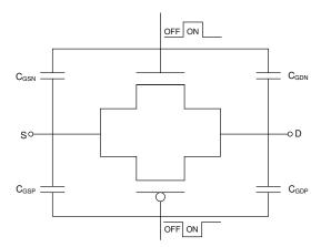
Figure 7-13. Transmission Gate Topology
