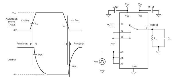
Figure 7-4. Transition-Time Measurement Setup
