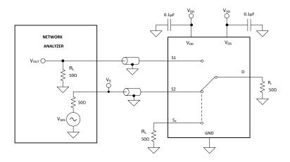
Figure 7-9. Crosstalk Measurement Setup
