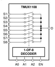
Figure 7-11. TMUX1108 Functional Block Diagram
