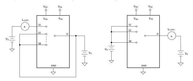
Figure 7-2. Off-Leakage Measurement Setup
