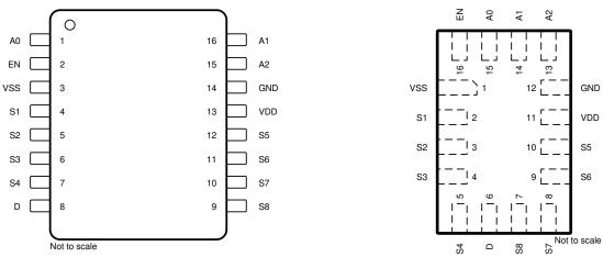
Figure 5-1. TMUX1108: PW Package, 16-Pin TSSOP (Top View)
