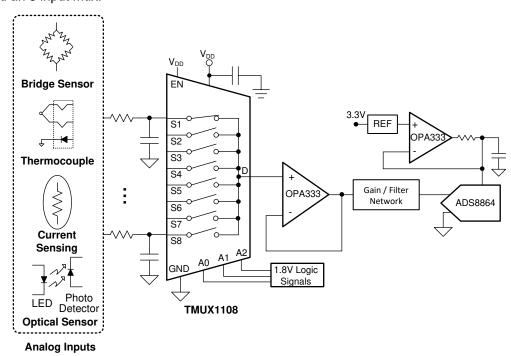
Figure 8-1. Multiplexing Signals to External ADC
