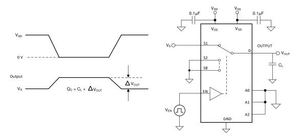
Figure 7-7. Charge-Injection Measurement Setup
