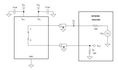
Figure 7-10. Bandwidth Measurement Setup
