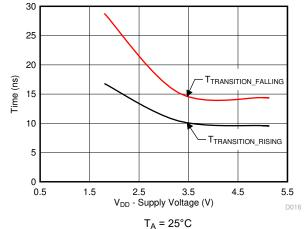
Figure 6-16. T<sub>TRANSITION</sub> vs Supply Voltage
