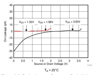
Figure 8-2. On-Leakage vs Source or Drain Voltage
