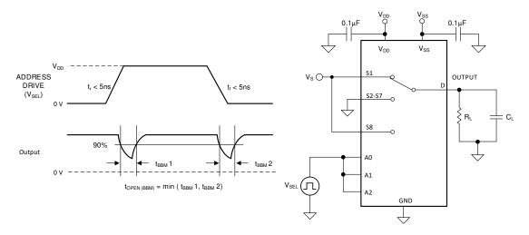
Figure 7-5. Break-Before-Make Delay Measurement Setup
