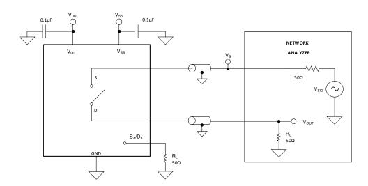
Figure 7-8. Off Isolation Measurement Setup
