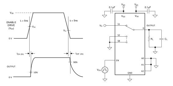
Figure 7-6. Turn-On and Turn-Off Time Measurement Setup
