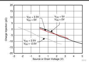
Figure 7-14. Charge Injection vs Source or Drain Voltage
