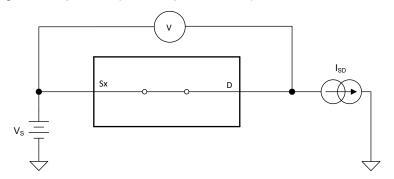
Figure 7-1. On-Resistance Measurement Setup
