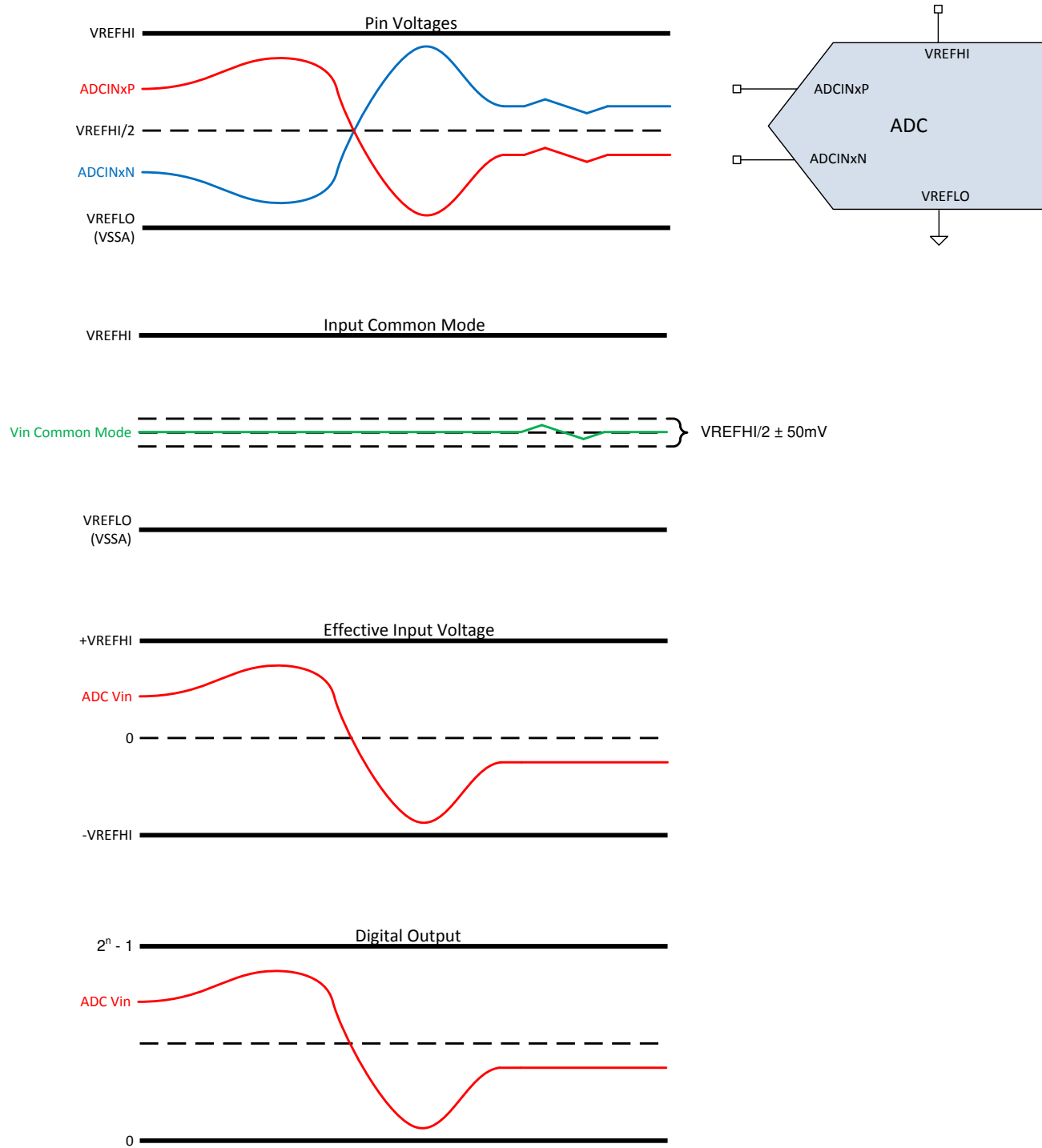
Figure 6-50. Differential Signaling Mode
