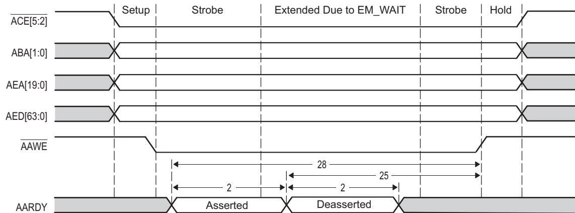
Figure 7-21 EMIFA EM_Wait Write Timing
