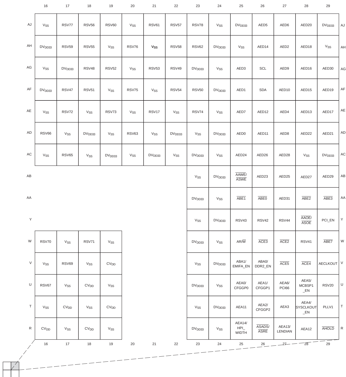
Figure 2-3. C6454 Pin Map (Bottom View) [Quadrant B]
