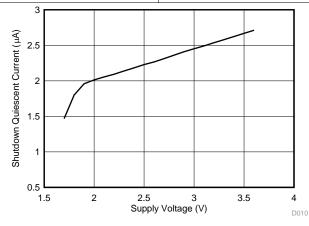
Figure 10. Shutdown Quiescent Current vs Supply Voltage
