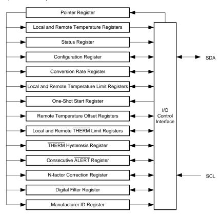
Figure 17. Internal Register Structure
