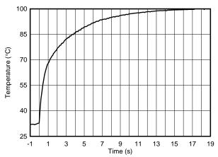
Figure 20. Temperature Step Response
