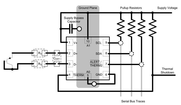
Figure 22. TMP461 Layout Example
