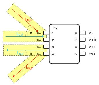
Figure 9-5. Magnetic Field Generated by Input Current Trace
