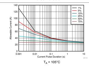
Figure 7-8. Maximum Repetitive Pulsed Current vs. | Figure 7-9. Maximum Repetitive Pulsed Current vs. **Pulse Duration**
