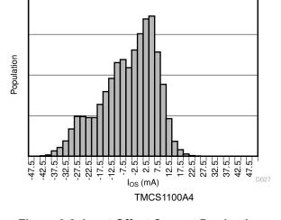
Figure 6-8. Input Offset Current Production Distribution
