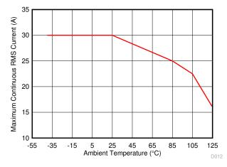
Figure 7-5. Maximum Continuous RMS Current vs Ambient Temperature
