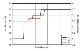
Figure 7-2. Transient Step Response
