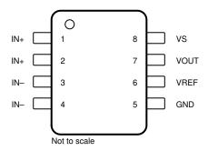
Figure 5-1. D Package 8-Pin SOIC Top View
