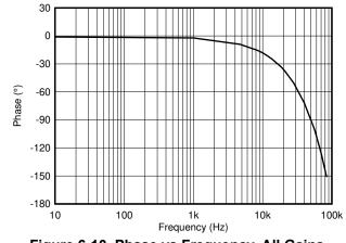
Figure 6-10. Phase vs Frequency, All Gains
