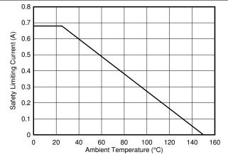
Figure 6-23. Thermal Derating Curve for Safety-Limiting Current, Side 2
