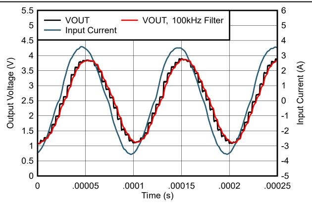
Figure 8-9. Response Behavior to 10kHz Sine Wave Input Current
