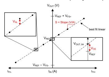
Figure 7-1. Sensitivity, Offset, and Nonlinearity Error
