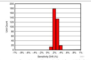
Figure 8-5. Sensitivity Error Drift After AEC-Q100 High Temperature Operating Life Stress Test
