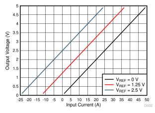
Figure 8-12. Output Voltage Relationship to Input Current With Varying VREF Voltages
