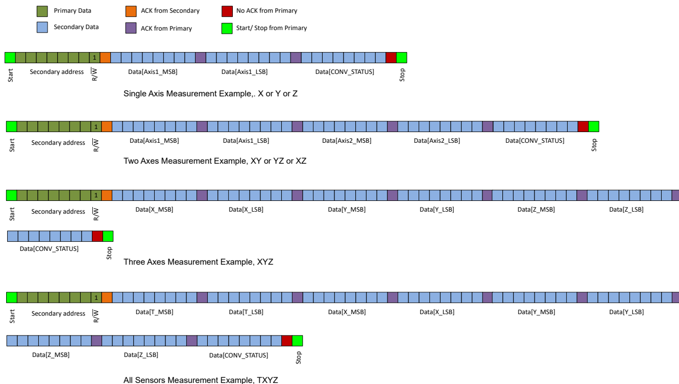
Figure 6-11. 1-Byte I 2 C Read Command for 16-Bit Data With CRC Disabled, CRC_EN = 0b
