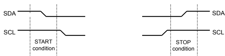
Figure 18-3. START and STOP Conditions
