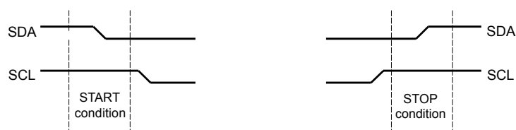
Figure 16-3. START and STOP Conditions
