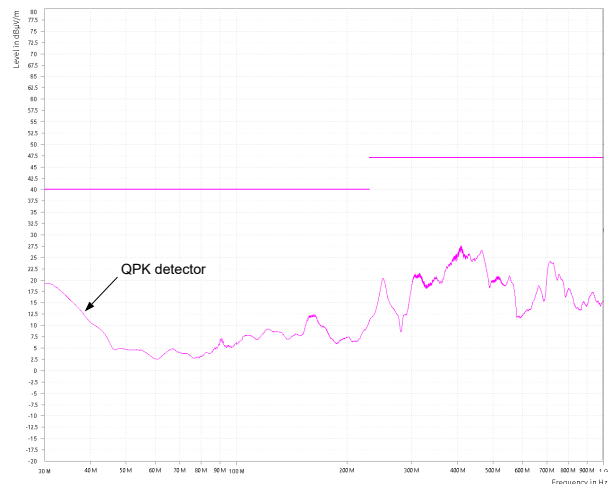
Figure 9-11. CISPR 32 Class B Radiated Emissions: Vertical Polarization
