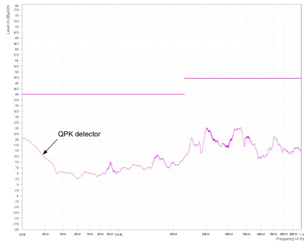
Figure 9-10. CISPR 32 Class B Radiated Emissions: Horizontal Polarization
