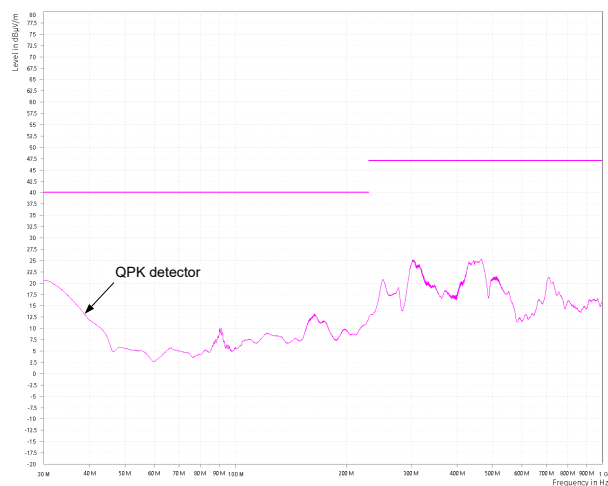
Figure 9-8. CISPR 32 Class B Radiated Emissions: Horizontal Polarization
