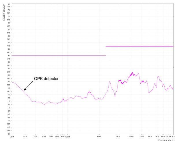
Figure 9-9. CISPR 32 Class B Radiated Emissions: Vertical Polarization
