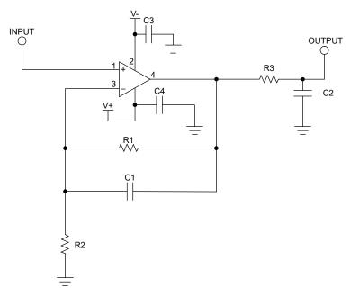
Figure 7-3. Schematic for Non-inverting Configuration Layout Example
