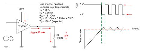
Figure 6-2. Thermal Protection
