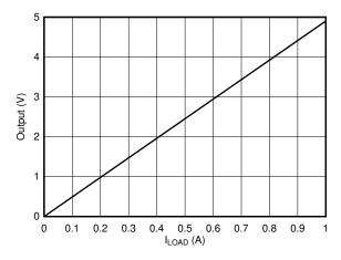
Figure 7-2. Low-Side, Current-Sense, Transfer Function
