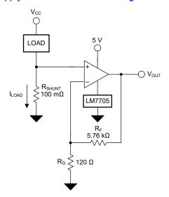
Figure 7-1. TLV936x-Q1 in a Low-Side, Current-Sensing Application
