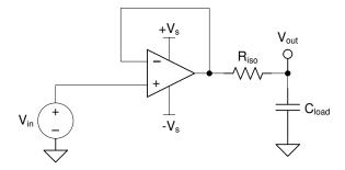
Figure 6-5. Extending Capacitive Load Drive With the TLV9361-Q1
