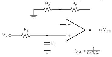
$$\frac{V_{OUT}}{V_{IN}} = \left(1 + \frac{R_F}{R_G}\right) \left(\frac{1}{1 + sR_1C_1}\right)$$
