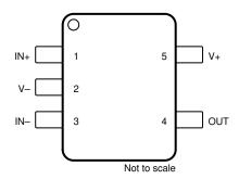
Figure 4-2. TLV9361-Q1 DCK Package 5-Pin SC70 (Top View)
