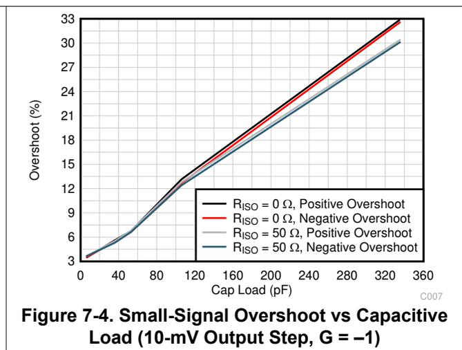
Figure 7-4. Small-Signal Overshoot vs Capacitive Load (10-mV Output Step, G = -1)
