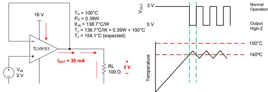
Figure 7-2. Thermal Protection
