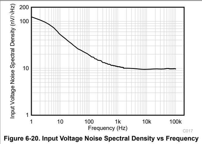
Figure 6-20. Input Voltage Noise Spectral Density vs Frequency
