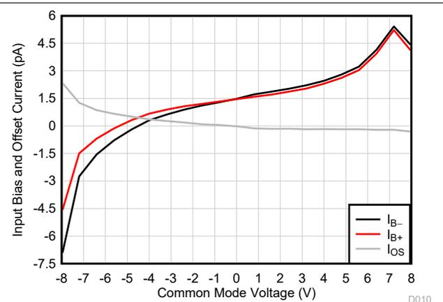
Figure 6-12. Input Bias Current vs Common-Mode Voltage
