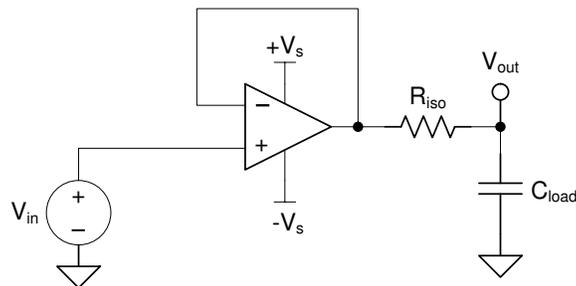
**Figure 7-5. Extending Capacitive Load Drive With the TLV9151**
