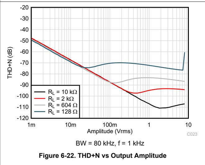
Figure 6-22. THD+N vs Output Amplitude
