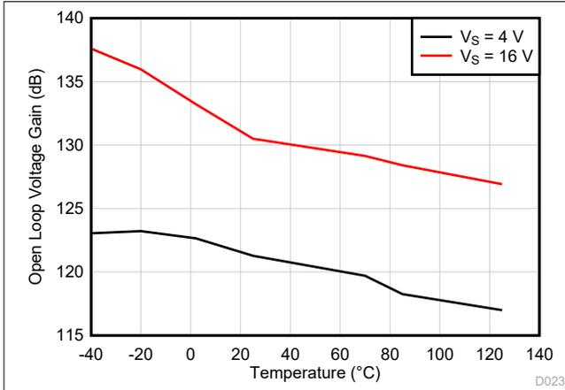
Figure 6-25. Open-Loop Voltage Gain vs Temperature (dB)
