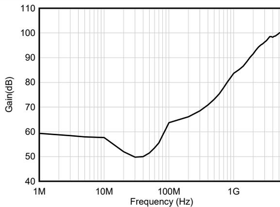
**Figure 6-41. EMIRR (Electromagnetic Interference Rejection Ratio) vs Frequency**
