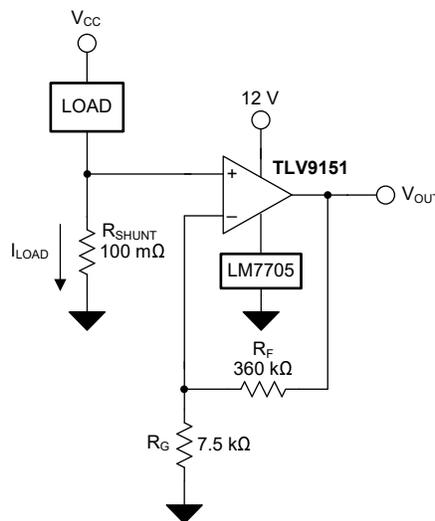
Figure 8-1. TLV9151 in a Low-Side, Current-Sensing Application
