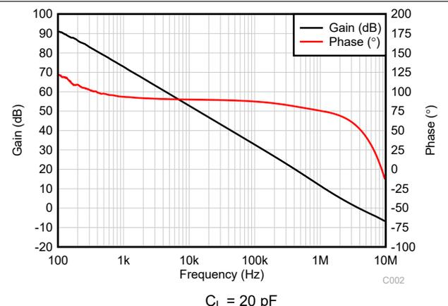
Figure 6-10. Open-Loop Gain and Phase vs Frequency
