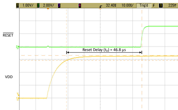
Figure 9-4. TLV841EVM RESET Time Delay ( t_D )
