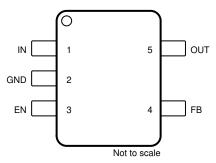
Figure 4-2. DBV Package, 5-Pin SOT-23 (Top View)
