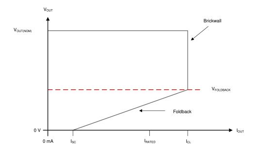
Figure 6-1. Foldback Current Limit
