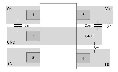
Figure 7-4. DBV Package (SOT-23) Typical Layout
