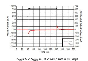
Figure 7-5. I<sub>OUT</sub> Transient From 250 mA to 850 mA
