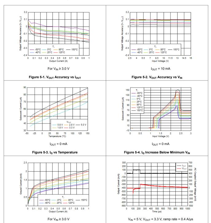
Figure 5-5. I<sub>GND</sub> vs I<sub>OUT</sub>
