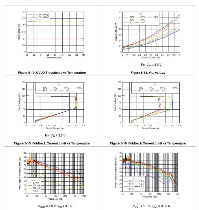
Figure 5-17. PSRR vs I<sub>OUT</sub>
