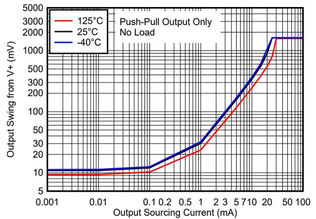
Figure 6-2. Output Swing vs. Output Sourcing Current - 1.8V
