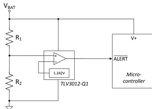
**Figure 8-3. Under-Voltage Detection**
