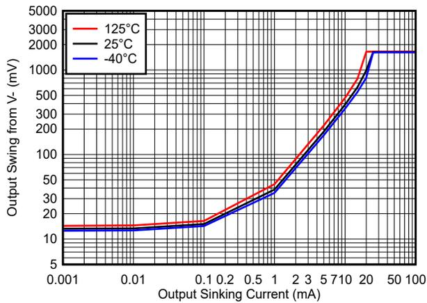
Figure 6-1. Output Swing vs. Output Sinking Current - 1.8V
