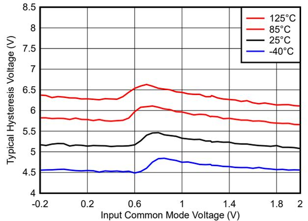
**Figure 6-22. Hysteresis Voltage vs. Common Mode, 1.8V**
