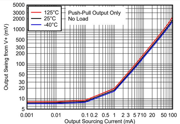
Figure 6-6. Output Swing vs. Output Sourcing Current - 5V
