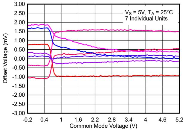
**Figure 6-31. Offset Voltage vs. Common Mode Voltage, 5V**
