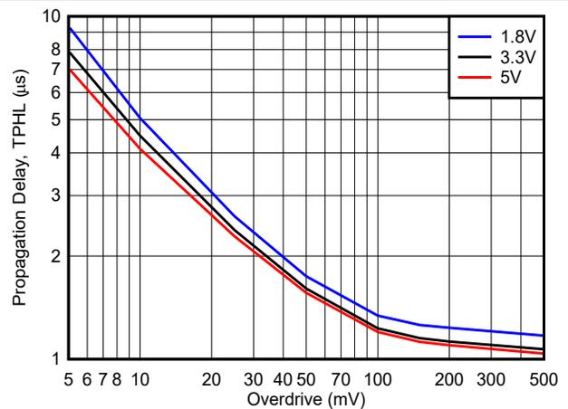
**Figure 6-12. High to Low Propagation Delay vs. Overdrive**
