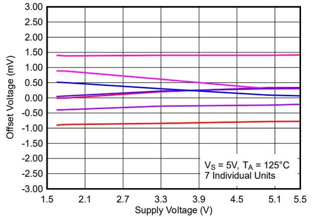
**Figure 6-32. Offset Voltage vs. Supply Voltage, 125°C**
