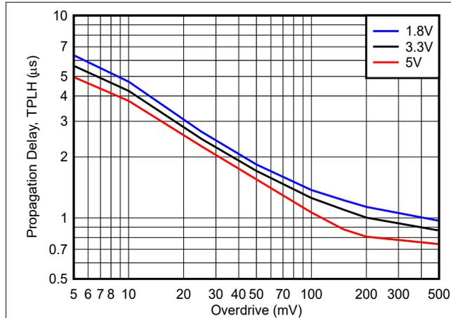
Figure 6-13. Low to High Propagation Delay vs. Overdrive
