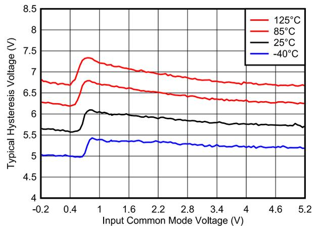
**Figure 6-24. Hysteresis Voltage vs. Common Mode, 5V**
