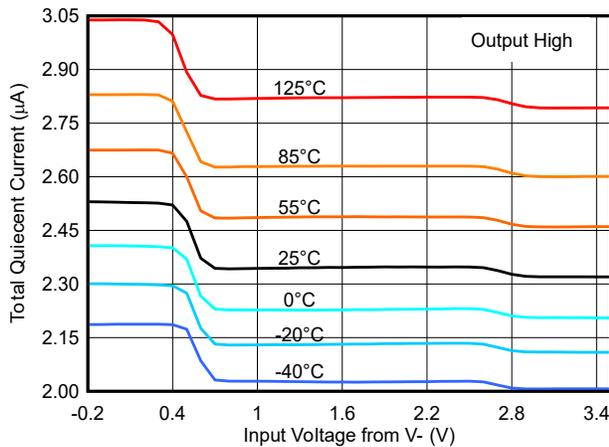
**Figure 6-9. Supply Current vs. Common Mode - 3.3V**
