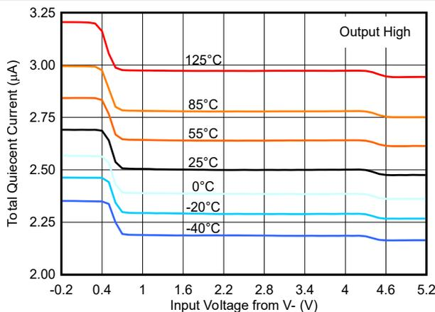
**Figure 6-11. Supply Current vs. Common Mode - 5V**
