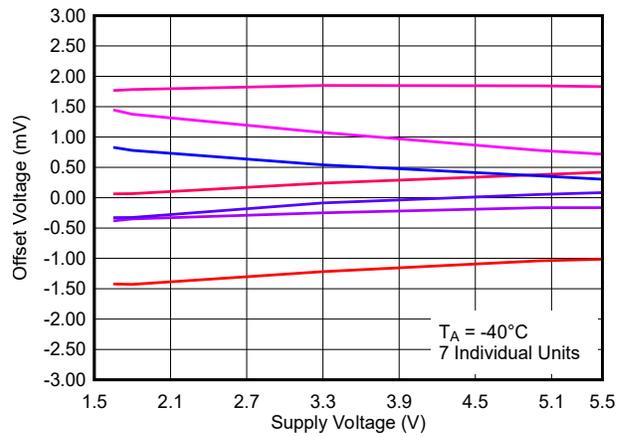
**Figure 6-34. Offset Voltage vs. Supply Voltage, -40°C**
