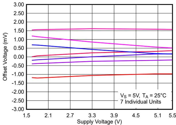
**Figure 6-33. Offset Voltage vs. Supply Voltage, 25°C**
