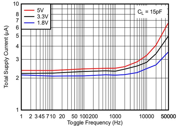
**Figure 6-20. Supply Current vs. Toggle Frequency - Push-Pull Output**
