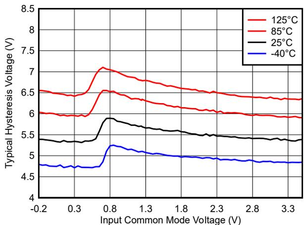
**Figure 6-23. Hysteresis Voltage vs. Common Mode, 3.3V**
