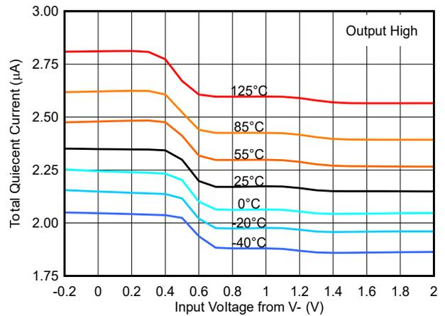
**Figure 6-10. Supply Current vs. Common Mode - 1.8V**
