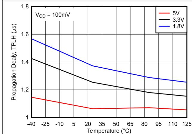
Figure 6-15. Low to High Propagation Delay vs. Temperature
