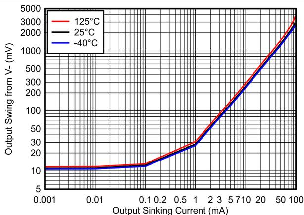
Figure 6-5. Output Swing vs. Output Sinking Current - 5V
