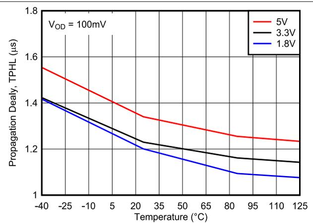
Figure 6-14. High to Low Propagation Delay vs. Temperature
