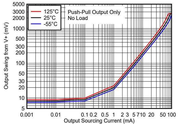
Figure 6-4. Output Swing vs. Output Sourcing Current - 3.3V
