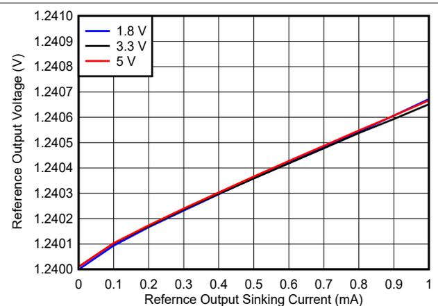
Figure 6-18. Reference Voltage vs. Reference Output Sinking Current
