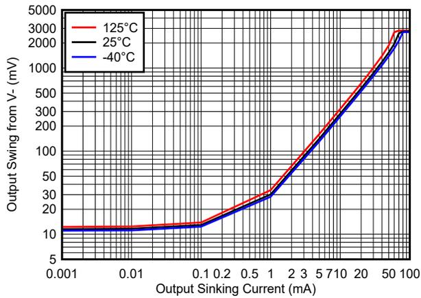
Figure 6-3. Output Swing vs. Output Sinking Current - 3.3V
