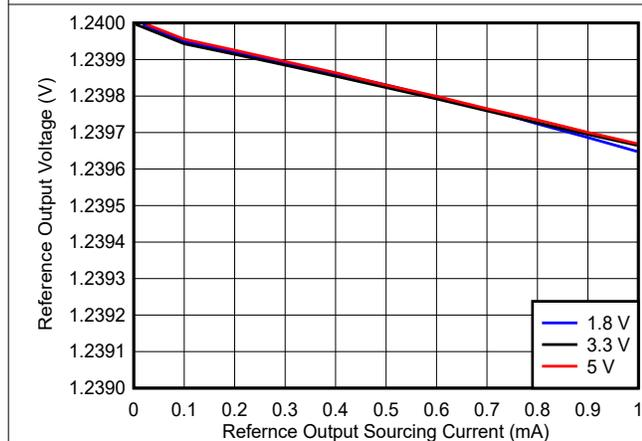
Figure 6-17. Reference Voltage vs. Reference Output Sourcing Current
