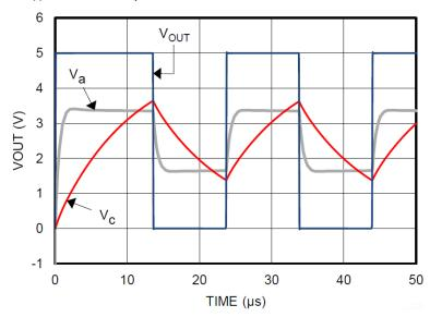
Figure 7-11. Square-Wave Oscillator Output Waveform
