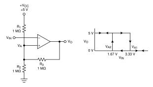
Figure 7-3. TLV183x in an Inverting Configuration With Hysteresis
