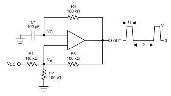
Figure 7-9. Square-Wave Oscillator
