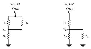
Figure 7-4. Inverting Configuration Resistor Equivalent Networks
