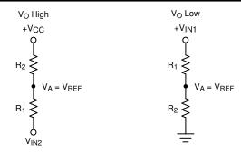
Figure 7-6. Non-Inverting Configuration Resistor Networks
