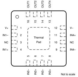
NOTE: Connect exposed thermal pad directly to V- pin.
