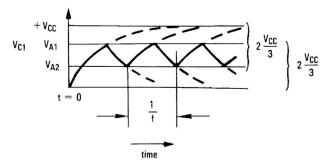
Figure 7-10. Square-Wave Oscillator Timing Thresholds
