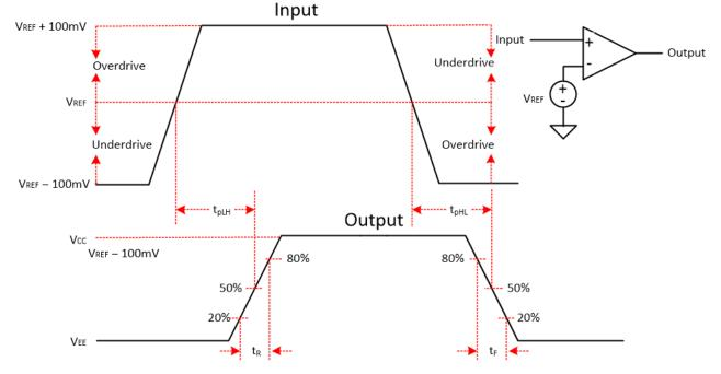
Figure 7-1. Comparator Timing Diagram
