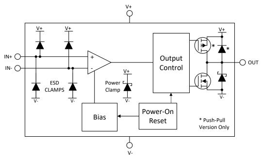
Figure 6-1. Block Diagram
