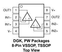
NOTE: Connect exposed thermal pad directly to V- pin.
