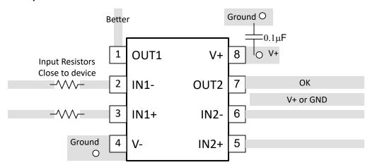
Figure 7-12. Dual Layout Example
