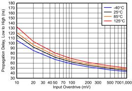
Propagation Delay, (Low to High) vs. Input Overdrive, 12V
