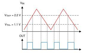
Figure 7-8. Window Comparator Results
