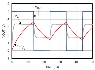
Figure 7-11. Square-Wave Oscillator Output Waveform
