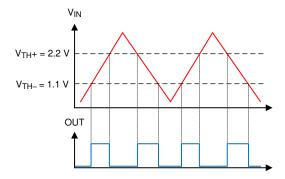
Figure 7-8. Window Comparator Results
