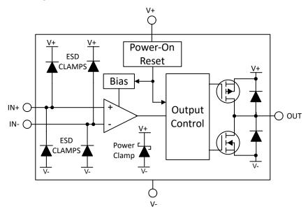
Figure 6-1. TLV1812-EP Block Diagram
