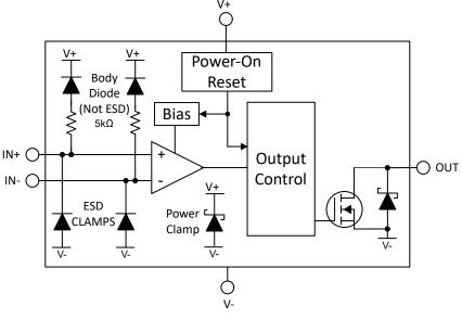
Figure 6-2. TLV1822-EP Block Diagram
