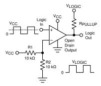
Figure 7-14. Universal Logic Level Shifter
