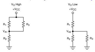
Figure 7-4. Inverting Configuration Resistor Equivalent Networks
